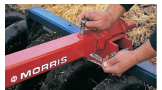
Universal Arm with quick detach pin for changing packers and harrows.
